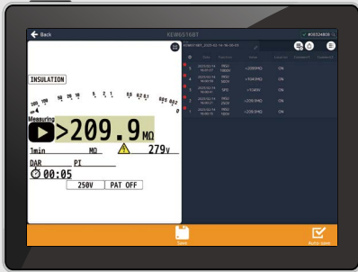
Real-time display and syncing data save on KEW Smart Advanced
